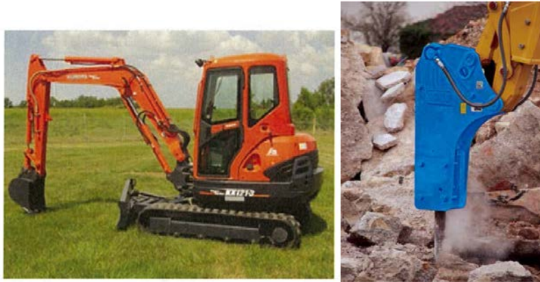
Figure 3-1: Excavator (KX121-3) and rock breaker attachment
