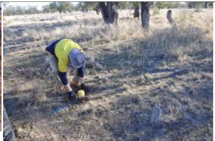
P.2 Installing the nodal geophones
