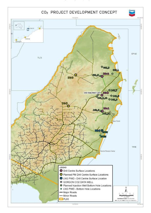
Figure 2.1: Overview of the drill centres associated with the propsoed Drilling and Completion Program
